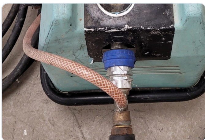
The inlet: a screw-collar coupling over a hose tail. Your hose clip keeps the hose on it.
