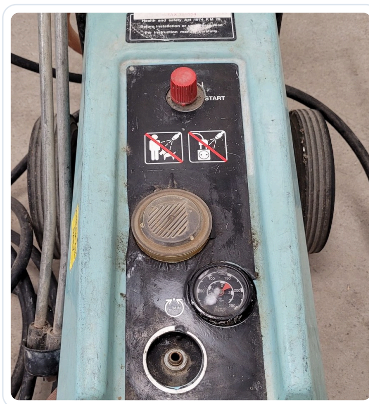
Top to bottom: red on/off knob, safety pictograms, oil sight glass, pressure gauge, water inlet.
